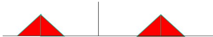
Figure.1 : Spectrum of the DSBSC wave
